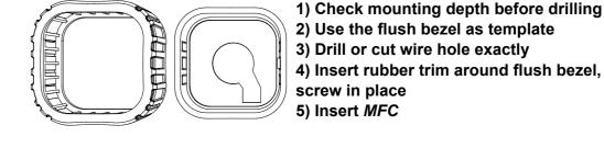
2) Use the flush bezel as template 3) Drill or cut wire hole exactly 4) Insert rubber trim around flush bezel, screw in place 5) Insert MFC
